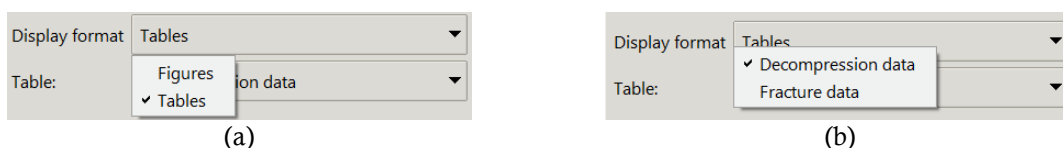
Figure 35 (a) Select the Table item of the Display format drop-down list from the Project panel to activate the module. (b) The module provides two types of tables: the Decompression data table and the Fracture data table .
