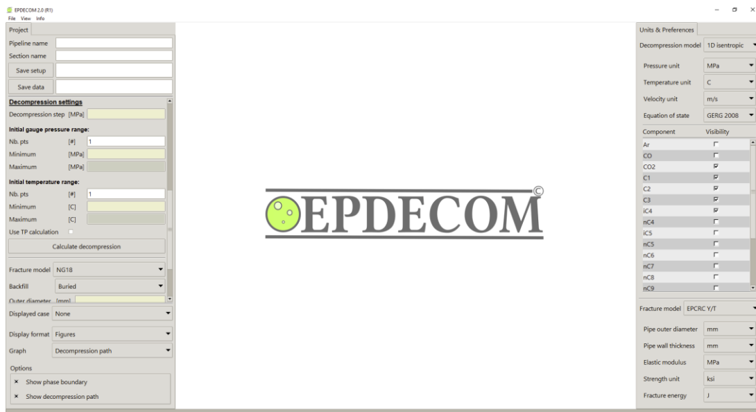
Figure 3 Main interface of EPDECOM V2.0 with the project panel on the left, the units and preferences panel on the right and the display panel at the centre presenting the EPDECOM logo.
