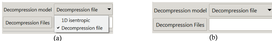
Figure 21 (a) Select the Decompression file model from the drop-down list of the Project panel. (b) The interface to the module is a single button and a text field listing the decompression files selected by the user.
