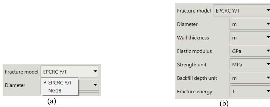
Figure 27 (a) Select the EPCRC Y/T model from the drop-down list of the Units & Preferences panel to access the module's preferences. (b) The preferences of the module.
