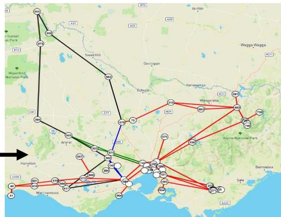
Figure 4: Our representation of the Victorian part of the NEM with the new transmission lines in green and the minor augmentations in black.
