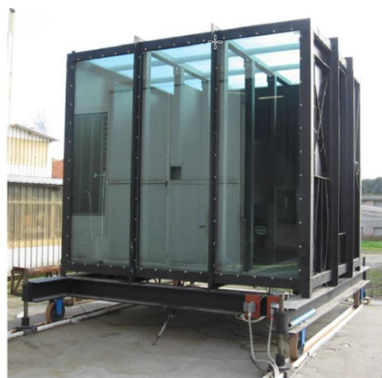
Figure 13: Photo of the Chamber View Explosion (CVE) test facility [18]
