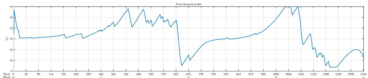
Figure 20: Profile of total linepack in the optimal hydrogen pipeline network in Victoria (see Figure 10).
