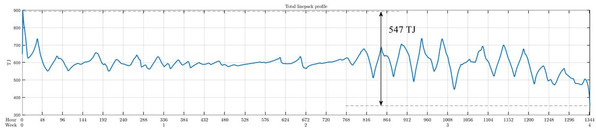
Figure 16: Profile of total linepack in the optimal hydrogen pipeline network in Queensland (see Figure 13) with the UHS in Roma. Note that the y-axis scale is from 300 TJ to 900 TJ.
