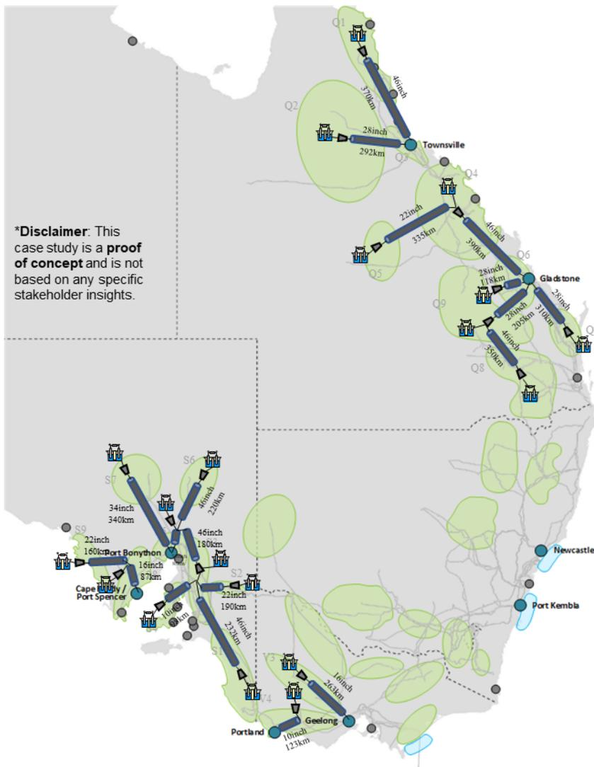
Figure 10: Optimal solution of the integrated infrastructure planning problem for the considered 2050 scenario. Only pipelines are deemed as the optimal transport infrastructure in this case study.
