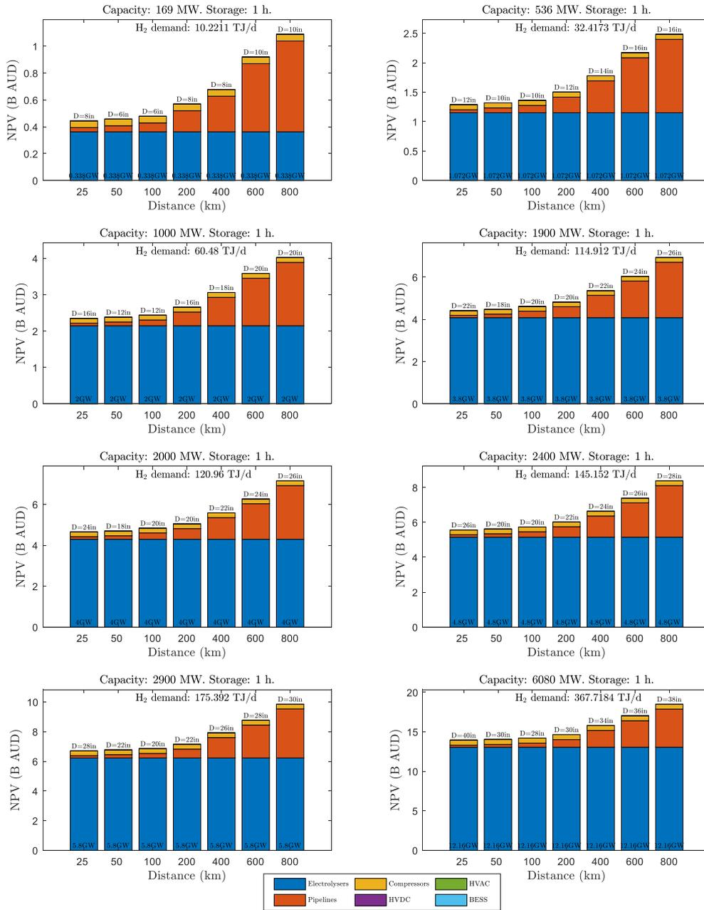
Figure 9: Optimal transmission and storage infrastructure across the considered capacities and distances, for a scenario requiring 1 hour of storage duration (Storage: 1 h), and with electricity options removed (only hydrogen pipelines are considered). Note the difference in y-axis scale between each case.
