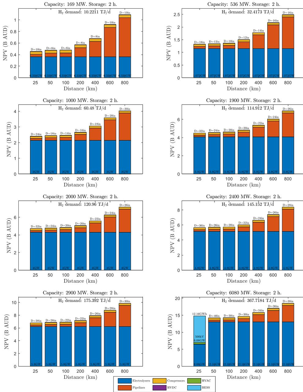
Figure 6: Optimal integrated transmission and storage infrastructure across the considered capacities and distances, for a scenario requiring 2 hours of storage duration (Storage: 2 h). Note the difference in y-axis scale between each case.
