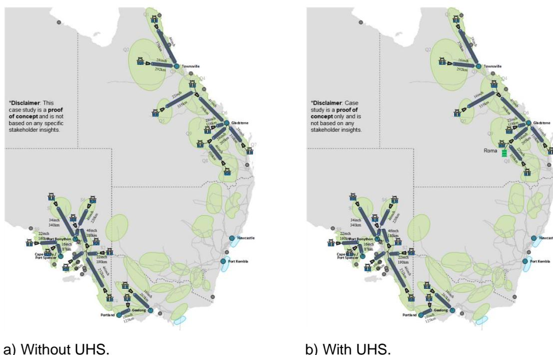
Figure 1: Optimal greenfield integrated infrastructure and storage designs for the two cases: a) without UHS, and b) with UHS. Notice the difference in pipeline diameters in Queensland between the two cases.
