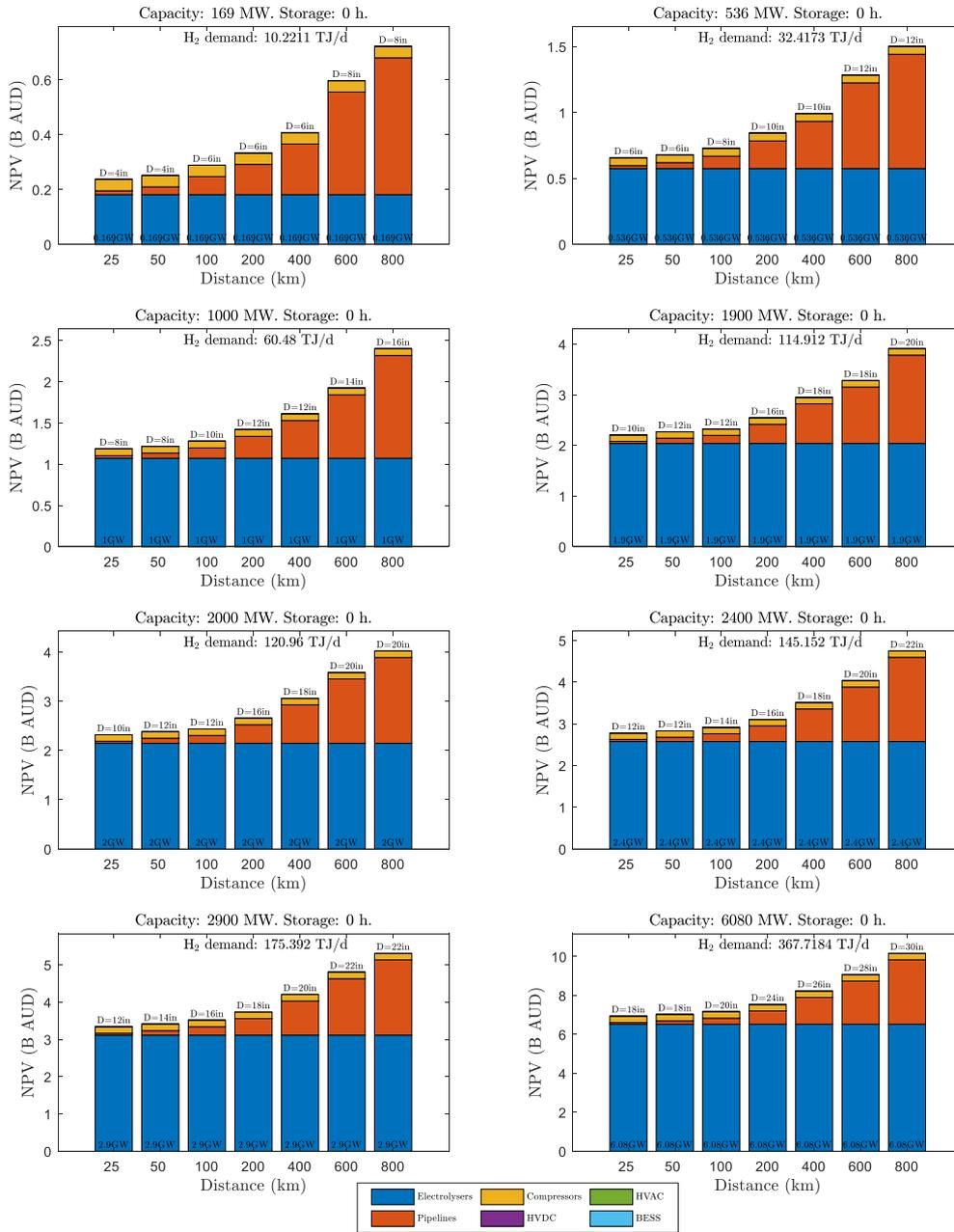
Figure 5: Optimal transmission infrastructure across the considered capacities and distances, for a scenario without storage (Storage: 0 h), i.e., where supply always exceeds the demand. Note the difference in y-axis scale between each case.
