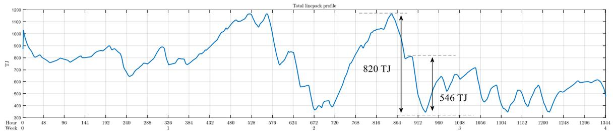
Figure 18: Profile of total linepack in the optimal hydrogen pipeline network in South Australia (see Figure 10).
