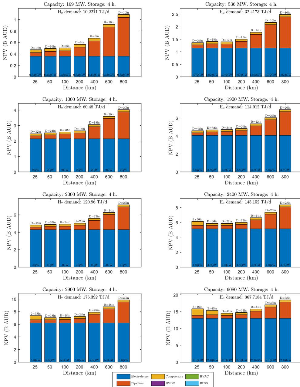
Figure 7: Optimal integrated transmission and storage infrastructure across the considered capacities and distances, for a scenario requiring 4 hours of storage duration (Storage: 4 h). Note the difference in y-axis scale between each case.
