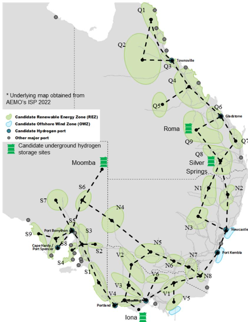
Figure 4: Dashed lines delineating the proposed provisional transmission corridors connecting REZ and hydrogen export ports. The figure also shows the proposed candidate UHS sites [19]. The underlying map is obtained from AEMO's 2022 ISP [1].
