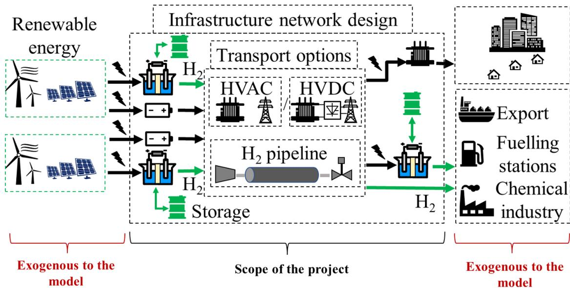
Figure 2: Illustrative scope of the integrated VRE transport and storage infrastructure model where the energy from multiple VRE hubs can be transported to a hydrogen demand hub using electricity lines and/or hydrogen pipelines over a network with arbitrary topology.
