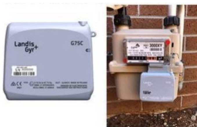
Figure 3 : Landis+Gyr Smart Dataloggers for monitoring gas usage of the 32 households
